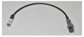
Fig 3 - Adapter For Computer Mic to Yaesu FT1000MP
