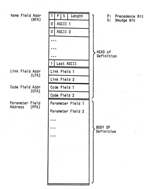
Fig. 4. Structure of a Definition
