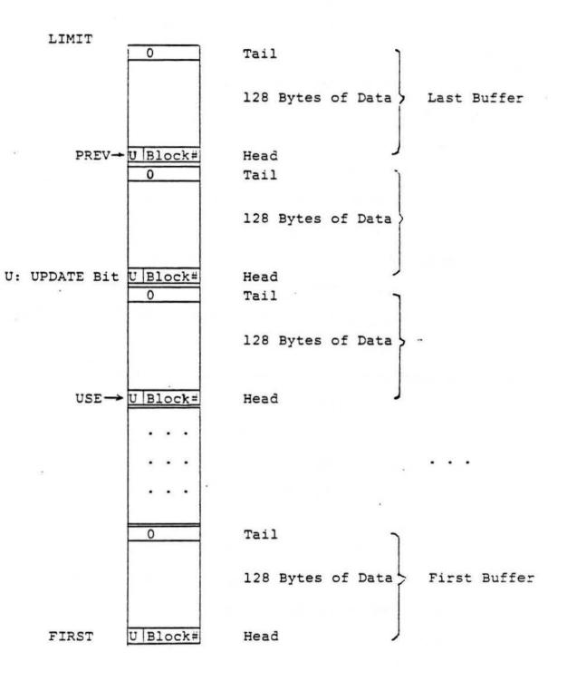
out of the disc is BLOCK . BLOCK calls another word BUFFER to look for an available buffer. BUFFER in turn calls a primitive word R/W to do the actual work of reading or writing the disc. These and other related words are to be discussed here. A flow chart of BLOCK is shown in Fig. 10 for better comprehension.
