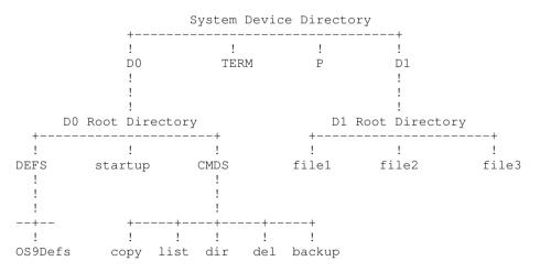
The device names in this example system are "TERM", "P", "D0" and "D1". The root directory of device "D0" includes two directory files, DEFS and CMDS, and one ordinary file "startup". Notice that device "D1" has in its root directory three ordinary files. In order to access the file "file2" on device "d1", a pathlist having two names must be used:
